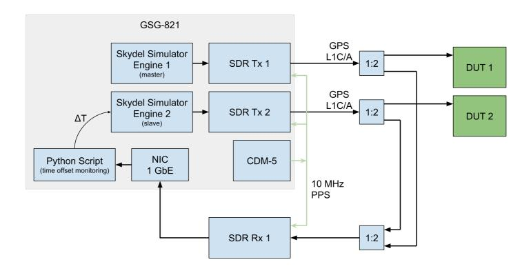
Orolia's Skydel Simulation software engine includes a rich API that allows customization without having to change the software itself. This solution runs with a standard software release and is enhanced by an external Python script and hardware to monitor a pilot signal that can measure the time offset and apply the correction.
